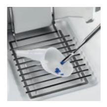
SmartPrep single-use, AntiStatic funnels provide a safe and fast method for weighing-in powders. Simply weigh, transfer and rinse. Fits nearly any standard 10–250 mL flask.
