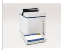
FastTrack™ UV/VIS technology comprises modern fiber optics in combination with array detection and a Xenon flash lamp for analyses within seconds. The instrument is always ready for use, as no time is required for warm-up.
