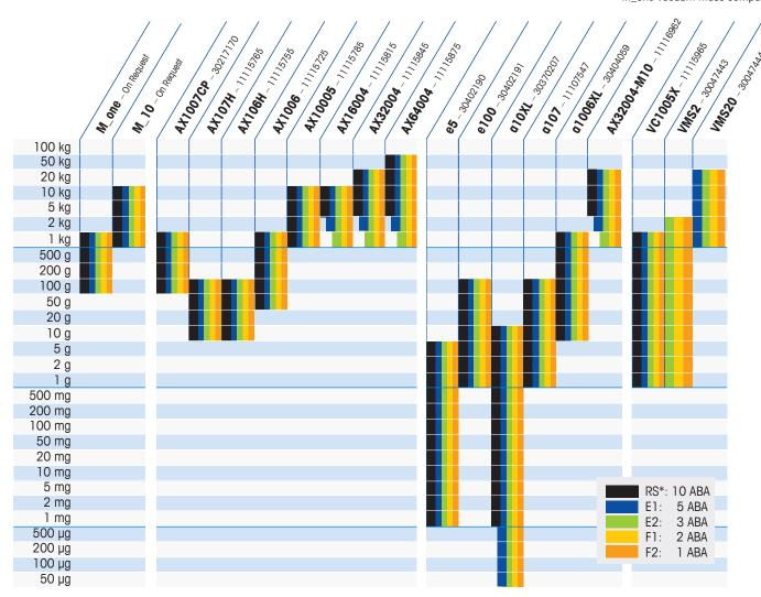
The illustration shows the application ranges according to the OIML R111 recommendation at zero meter-altitude. In cases where the application range is limited by the physical size of the weight, additional support plates may be required to accommodate smaller weights. Please contact us for a personal consultation to discuss your individual needs.
