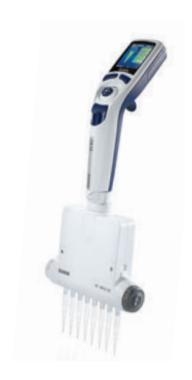
E4 XLS spacers let you set nozzle spacing for 24-, 48- or 96-well plates with just a twist: 9–19 mm on 6-channel and 9–14 mm on 8-channel models. The liquid end rotates 360° for quick alignment with the plate. E4 XLS spacers are ideal for genomic, proteomic and cell-culture applications.
