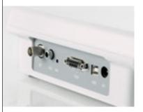
FiveEasy™ Plus series meters allows data to be exported either directly to a printer or PC for further processing using its RS232 or USB ports.
