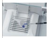
SmartGrid™ minimizes the effects of air currents to dramatically reduce stabilization times. Spilled substances fall through the grid and do not influence your weighing results.
