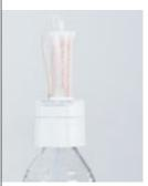
The solvent manager takes care of filling, draining and exchange of reagents. It is controlled by the titrator and full security is guaranteed by the overflow protector in the waste bottle.
