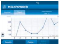
Define up to 20 methods using standard or rapid drying with various switch-off criteria and display units. Store up to 100 results in the instrument and review them easily in the results overview. Either print your results or transfer them to an USB flash drive or PC.
