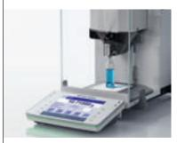
This gravimetric sample preparation uses precise balance results to produce accurate concentrations, in contrast to error-prone visual readings when using volumetric flasks. Automatic results recording also eliminates transcription errors.
