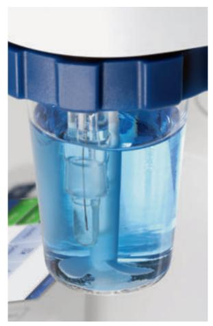
G20S with manual titration kit and DGi115-SC in a glass titration beaker
