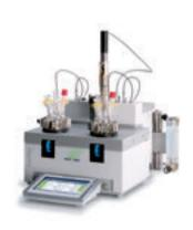
EasyMax makes chemical synthesis easier by eliminating the dependence on ice baths, oil baths, and chillers. Quickly explore reaction conditions, even under low temperatures, while recording data that would otherwise be missed.
