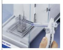
AntiStatic Kits completely remove electrostatic charges. The scattering of powdery substances is eliminated, making dosing safer and preventing cross-contamination.
