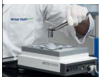
Balance calibration is at the core of accurate results. Our GWP Verification service proves balance accuracy on-site and includes an optimal routine testing/calibration schedule, specification of required test weights, and the ideal maintenance plan.
