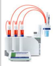
The T7 is a titrator for any application including multitasking, flexible method-editing, upgradeability (additional pH-sensor or conductivity board for T9 functionality) and method loops for the integration of various methods into one or more sample series sequences. It is a flexible and expandable system that adapts easily to current and future needs.
