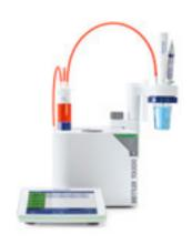
The T5 titrator is a ready-togo-system capable of general potentiometric titration, as well as volumetric and coulometric Karl Fischer titration, for users who need a simple, rugged and easily-understandable titrator for fast routine analyses. The T5 offers top-of-the line features such as SmartSample™, an error-free data transfer of your sample information from the balance to the titrator, and StatusLight™, which checks the status of your titrator in a fast, simple and intuitive way.
