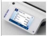
Eight embedded applications including check-weighing, totaling and formulation simplify daily tasks. The statistics option lets you easily evaluate your weighing results.
