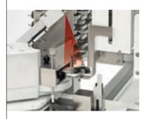
The integrated data-matrix-code scanner automatically identifies the filter ID and ensures fast and easy operation. Sample security before and after processing is maintained.
