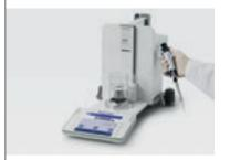
All test data is stored safely on a built-in RFID chip on RAININ pipettes, or a Smart Tag can be added for other pipette brands. The balance application guides you through the testing process. Use an evaporation trap for the most accurate results.
