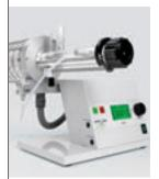
The manual Karl Fischer DO308 drying oven allows safe oven applications with single samples using manual sample addition. It can be operated with both coulometric and volumetric Karl Fischer titrators.
