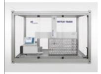
Our e\_Line and a\_Line mass comparators carry out weight calibration in a fully automated process, significantly reducing calibration times and measurement uncertainty.
