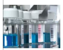
LiquiPhysics™ Excellence is not only able to read barcodes; it can also accurately interpret their information. With Smart Codes containing information about the type of product to be measured, the user simply scans the barcode to start the measurements. There is no additional button to click.
