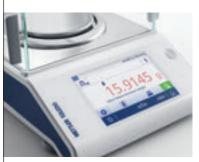
The weight value remains red until the net sample weight is above the pre-programmed minimum value. A user-defined minimum weight can also be programmed into the balance to provide an additional safety factor.
