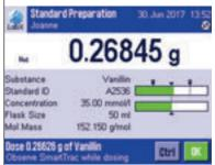
LabX laboratory software provides flexible SOP user guidance on the balance's touchscreen.
