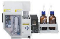
SC automation units are available in heated versions suitable for performing density measurements of samples which are highly viscous or even solid at ambient temperature such as paraffins, bitumen, heavy crude oils and edible fats. The SC1H and the SC3OH can handle samples with a melting point of up to 60 °C.
