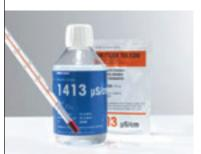
Depending on the type of sensor, conductivity standards are used for calibration or verification.
