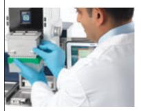
Quickly replaceable liquid heads provide great flexibility. Get the precision you demand with the 0.5–20  $\mu$ L head, the daily workhorse you need with the 5–200  $\mu$ L head and the multidispensing capability of the 100–1,000  $\mu$ L head.
