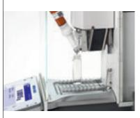
Powders are sealed within the dosing head. Individual dosing heads for each powder eliminate the risk of cross-contamination. Once the dosing head is filled, work proceeds with no powder contact.
