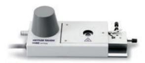
Hot-Stage microscopy is a powerful tool that is widely used for the visual characterization of all kinds of thermal transitions. The possibility of directly observing morphological changes in a sample as it is heated or cooled is of enormous value. Changes in the shape, structure and color of crystals are seen as well as their size and number. The technique allows phase transitions to be characterized and provides information on expansion and shrinkage behavior.
