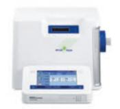
DM density meters determine the density and/or specific gravity of liquids quickly and accurately. The results are automatically converted into one or several pre- or user-defined units such as Brix, API degrees or alcohol concentrations. Automatic error detection, entire temperature range adjustments and built-in algorithms shorten measurement times required by up to 75 % — DM and DX are doubtlessly the state-of-the-art pinnacle for digital density measurement.
