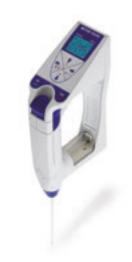
The Densito 30PX and the Refracto 30PX offer all the features required for successful on-site density and refractive index measurements including automatic temperature compensation, direct display of the result in the desired unit, built-in timekeeping for full GLP compliance and data output via infrared interface. Densito and Refracto come with practical carrying cases which contain everything necessary to carry out measurements.
