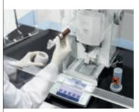
Potent or toxic compounds remain sealed within the dosing head and hence aerosol formation is kept to a minimum. With an automated dosing process, users work safely without exposure to substances during weighing.
