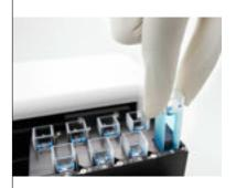
This auto-changer offers you efficient automatic measurement of series of up to eight cuvettes for both standard measurements with blank subtraction or complex kinetic applications, thermostatable from 10 °C to 80 °C.
