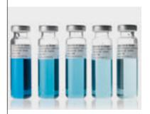
Prepare concentrations down to 0.1 mg/g in one step in accordance with USP. Automated liquid dosing delivers precise concentrations every time because solvent is added automatically based on the actual weight of weighed-in solids.
