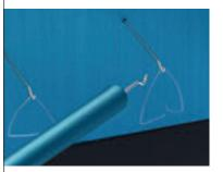
Precise and inimitable shapes for each nominal weight. To ensure accuracy, an automated process is used to bend wires with diameter as small as 0.05 mm into desired shapes.
