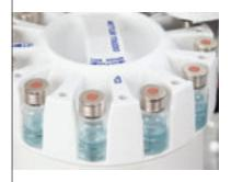
After quenching, the liquid handling system dilutes the sample to a user specified concentration and transfers it to a vial, ready for offline analysis. Quench and dilution steps can function as sample derivatization steps, thus decreasing sample preparation time and eliminating human error.
