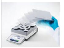
The SmartPan™ weighing pan minimizes the effects of air currents on the weighing cell to deliver faster and more accurate results. In most conditions a draft shield is no longer needed, significantly reducing process steps.
