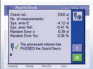
The XPE balance comes standard with easy-to-use, step-by-step guidance. Based on ISO 8655, it calculates all results automatically and shows pass/fail decisions.
