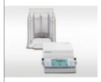
Achieve the smallest uncertainties possible on manual comparators with AX window-range models. Hanging weighing pans, double draft shields and sophisticated weighing cells secure the best results for higher weight classes.
