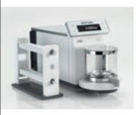
By neutralizing electrostatic charges on samples and containers when the balance is loaded, dosing is faster and productivity is increased.
