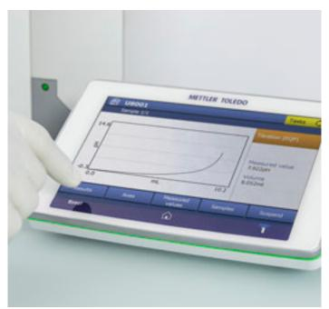
Intuitive user guidance and a brilliant color touchscreen makes operation simple. Save up to 24 method or manual operation shortcuts that can be started with One Click<sup>TM</sup>. Plug a USB stick for easy downloading of PDF reports in seconds.
