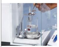
The built-in application on XPE and XS balances provides user guidance, collects results, calculates density values and allows statistical evaluation of a measurement series. Five methods are included.
