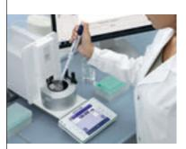
The Calibry-Software cockpit screen ensures efficient pipette calibration workflows in accordance with ISO 8655. User management, audit trail and a secure database help ensure compliance with FDA 21 CFR Part 11.
