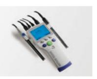
The large SevenGo Duo display shows all relevant setting and highlights the most important items. You can read the measurement value and check the state of the electrode at a glance. The results of parallel measurements appear in an alternating fashion on the display.
