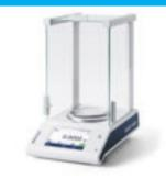
Capacity up to 320 g Readability 0.1 mg Minimum weight 16 mg USB minimum weight 160 mg
