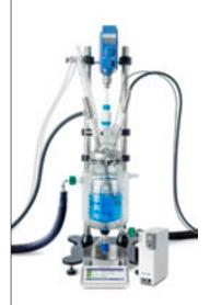
Connect and control your jacketed laboratory reactor with programmable temperature, liquid dosing and sampling for data-rich experiments, day or night. Automation and data capture allows researchers to scale-up more successful experiments.
