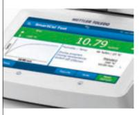
Simply select the integrated SmartCal method on the instrument, distribute the contents of the test sachet evenly over the sample pan and start the measurement. After ten minutes, you know if your instrument's performance is satisfactory or not.
