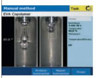
Observe your measurements in real time via video or replay the video to verify your results. Digital image analysis and automatic detection of dropping and softening points guarantee that results are reliable.
